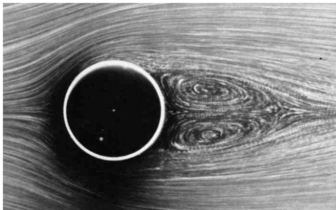
Figure 2: Photograph by Sadatoshi Taneda a cylinder moving through a tank of water. The flow is visualized using aluminum powder. The image is taken from An Album of Fluid Motion by Milton Van Dyke, Parabolic Press, 1982.
